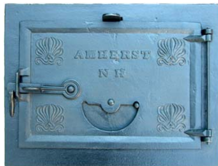
1.30 Cast iron bake oven door unit made in Amherst, N.H. The pull-tab at the top operates a built-in damper, and the vent is weighted to stay in the open position.
